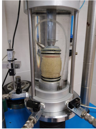
Figure 7. Silica sand sample subjected to pressure in a triaxial cell.
