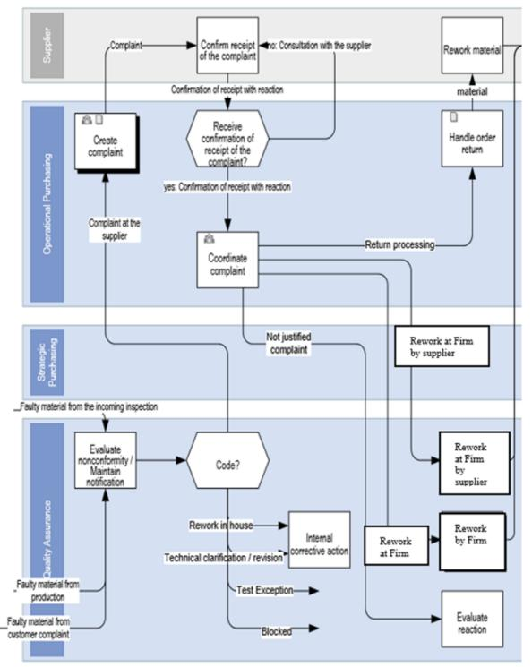
Figure 2. Supplier complaint process flow (Medina-Serrano, 2019)
