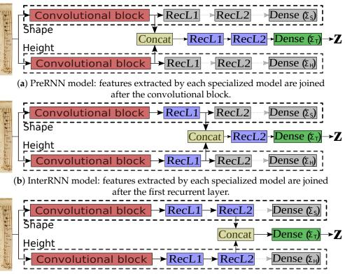
(c) PostRNN model: features extracted by each specialized model are joined after the recurrent block.
