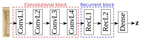
Figure 2. Graphical scheme of the CRNN configuration by Calvo-Zaragoza et al. [20].
