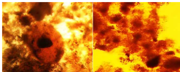
Figure 2 | Structure of anaerobic granular sludge of recent formation in UASB stage (×10).
