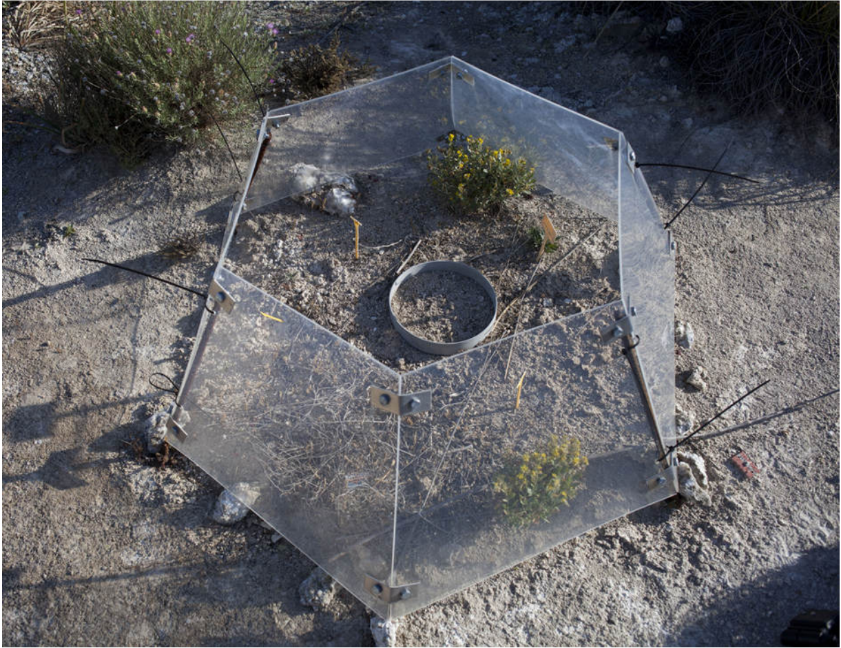
Supplementary Figure 6 | View of an experimental plot of the warming treatment in the field experiment.
