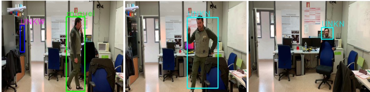
Fig. 14. Random results of the proposed approach with the bounding box and the predicted identification of the person superimposed. Boxes and texts in green mean a hit with known people. Blue boxes and texts mean they have been classified as unknown. In the first example, it can be seen that the body detector has identified a reflection on the glass as a person, but the proposed system has managed to identify it as unknown. The following examples show the potential problems of the system, the partial or total occlusion of the body. These examples will be discussed later in the Limitations section.
