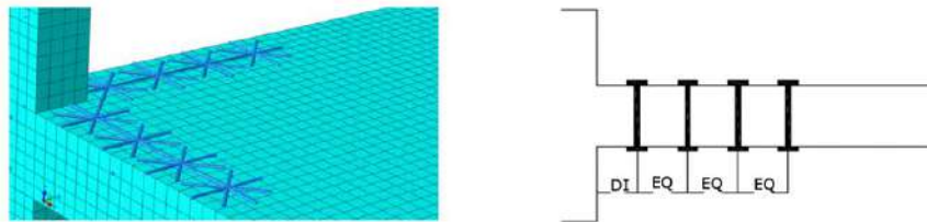
Figura 3. Shear bolt arrangement in the slab model simulating retrofitted in [2]. Left: general view of the FEM. Right: diagram showing location and spacing of shear bolts.
