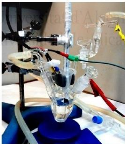
Figure 2.1. Electrochemical cell of three electrodes.
